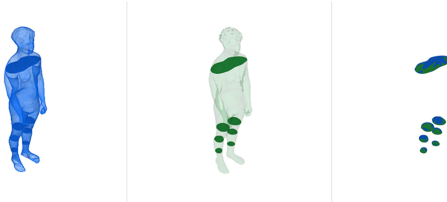
Figure 8 Basic body measurement comparison. Left: First 4D-scanner frame with slices (darker blue); Middle: Turntable scanner frame with slices (darker green), Right: Slices superimposed onto each other.
