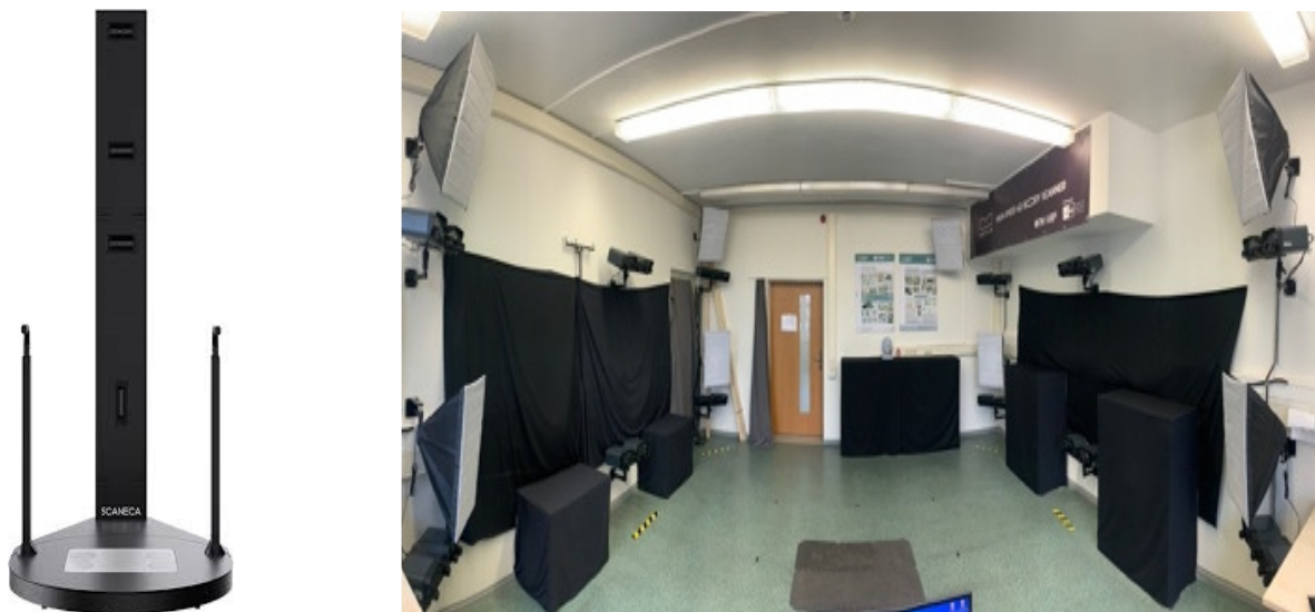
Figure 2 Scanning systems used in the experiment. Left: Scaneca turntable 3D-scanner; Right: MOVE4D multimodule 4D-scanner at TUD Dresden University of Technology
