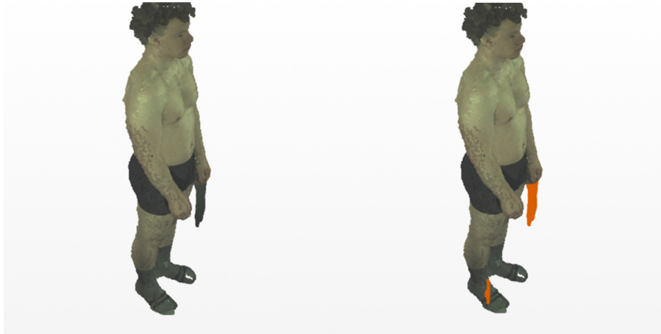
Figure 3 Cleaning fragments of the scanner out of the pointclouds. Left: Original pointcloud frame. Right: The same pointcloud frame, the points marked for disposal are highlighted in orange.
