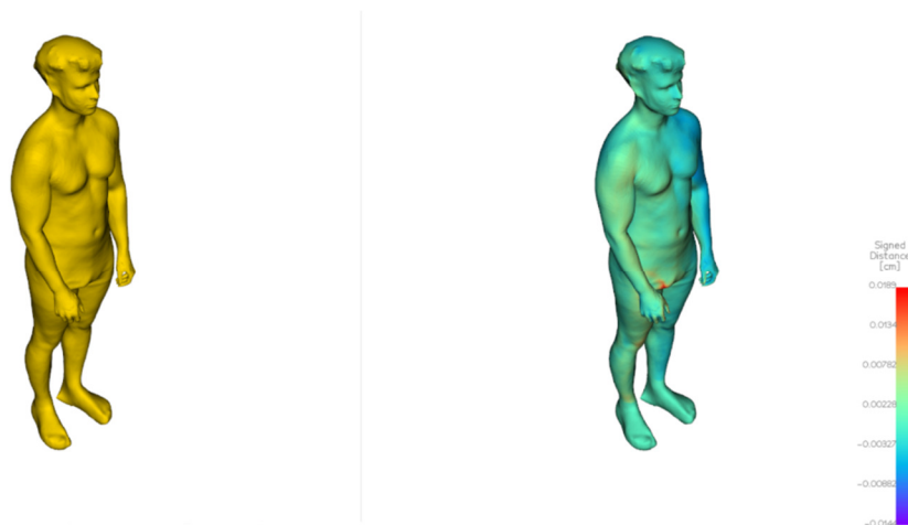
Figure 1 Left: Third frame of the 4D-scan. Right: Third Frame of the 4D-scan, rotated & translated to the first scan position. The colors show the movement between this frame and the previous one.
