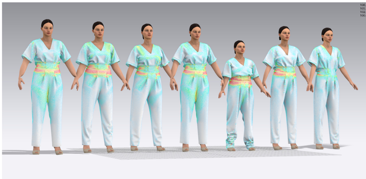
Fig. 6. Stress map showing the distortion of the reference size 12 garment when fitted 7 avatars.
